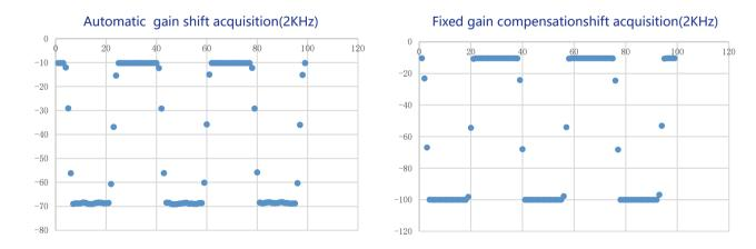
The fixed gain compensation setting has a shorter response time for large dynamic range data acquisition
